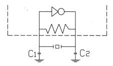
Load capacitance ( $C_L$ ), which is specified in picofarads (pF), can be calculated by the following formula:
