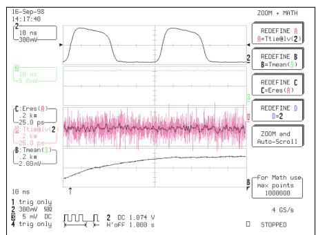
Figure 1 – Using Trend of Time Interval Error@Level to verify the temperature stability of a clock oscillator
