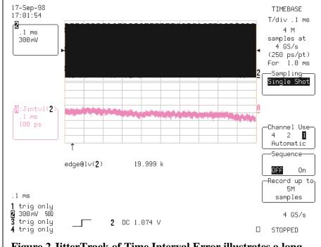
Figure 2 JitterTrack of Time Interval Error illustrates a long term change in oscillator period over a 1 ms acquisition time
