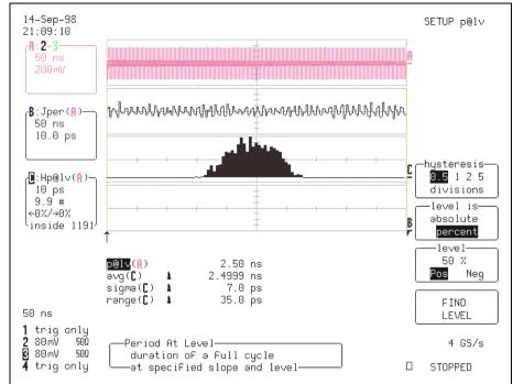
Figure 3 – A jitter measurement of a 400 MHz oscillator taken over 1191cycles of the clock period with a LeCroy scope
